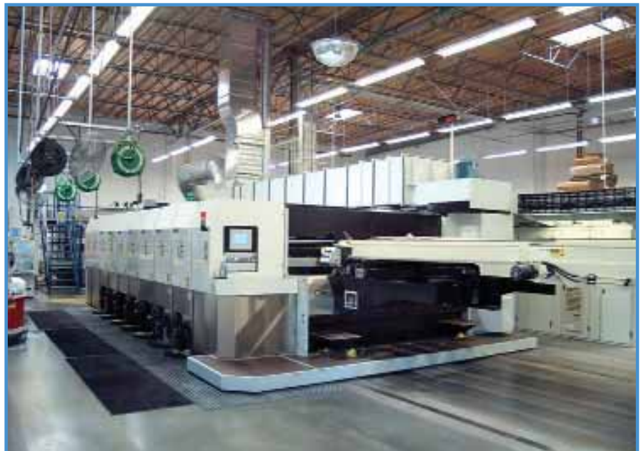
Allpak's DRO is a six-color-plus UV vacuum transfer rotary die cutter that is capable of running at speeds of 11-thousand sheets per hour, while maintaining two-tenths of a millimeter register from color-to-color.
